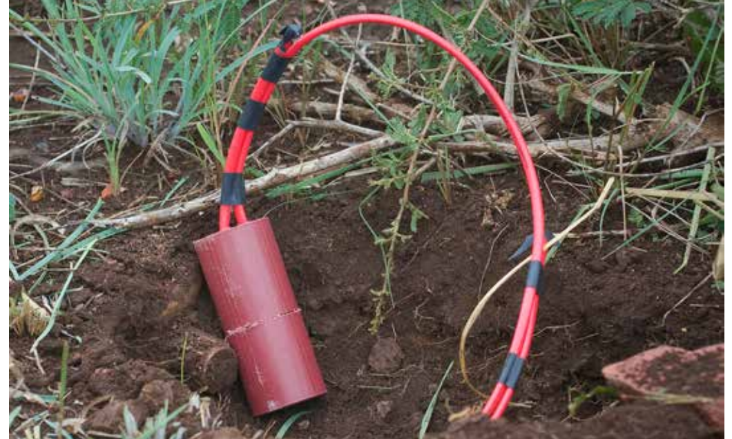
A pentolite fuse and charge laid next to a Russian Federation Antipersonnel Blast Mine.
